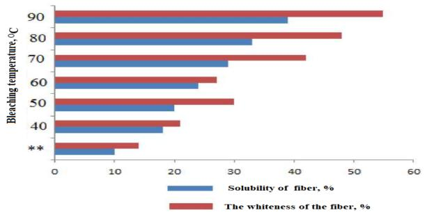
Bleaching and discolouring processes of washed white, yellow, cream, blue and brown wool fibers were carried out. The composition of the solution consists of hydrogen peroxide as a bleach, sodium silicate as a stabilizer and SAMs of various activities.
