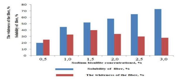
used as the main reagent in the solution when bleaching wool fibers with the help of reducing agents. Bleaching in bisulfite solution was carried out at room temperature for one day in 0.5-3.0% sodium bisulfite solution with a modulus of 20. The fibers were then compressed and treated with a solution of sulfuric acid (5% by mass) for 15 minutes, then washed with water. The results of a study on bleaching of wool fiber under the influence of reductants are shown in Figure 2.
