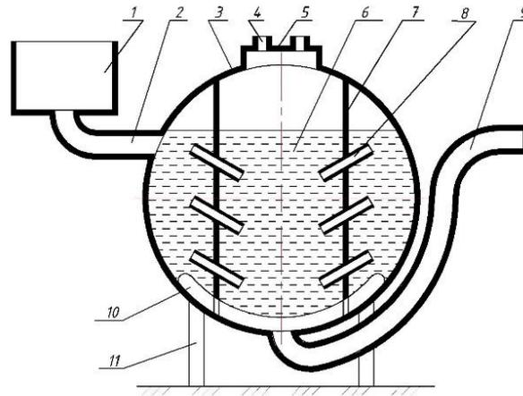
Fig.1. Experimental production plant for anaerobic processing of organic waste of birds.
